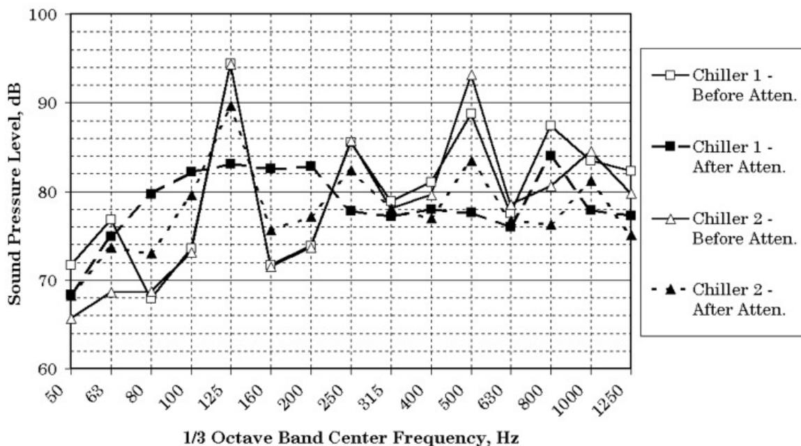
**Figure 1:** Air Cooled Chiller Compressor Noise; Helical Rotary (Screw Compressor, with Attenuation VS without; Measurements taken @ 1m.
