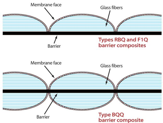
Mass-loaded quilt can be used to jacket noisy compressors, if thermal considerations allow it.
