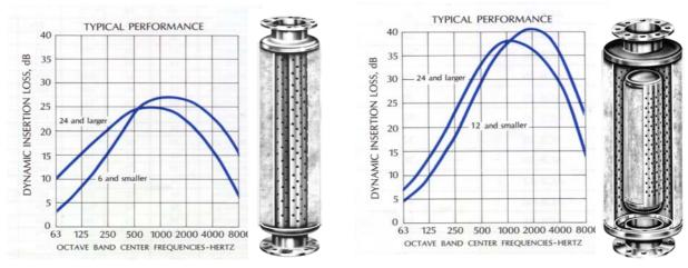
Others have a greater diameter inner wall, with a perforated "bullet" insert inside the pipe. These can have somewhat greater attenuation, but at the cost of slightly greater pressure drop. Both variations have good mid- to high-frequency attenuation, but poor low frequency attenuation. (Illustrations courtesy of Burgess Manning<sup>6</sup>)
