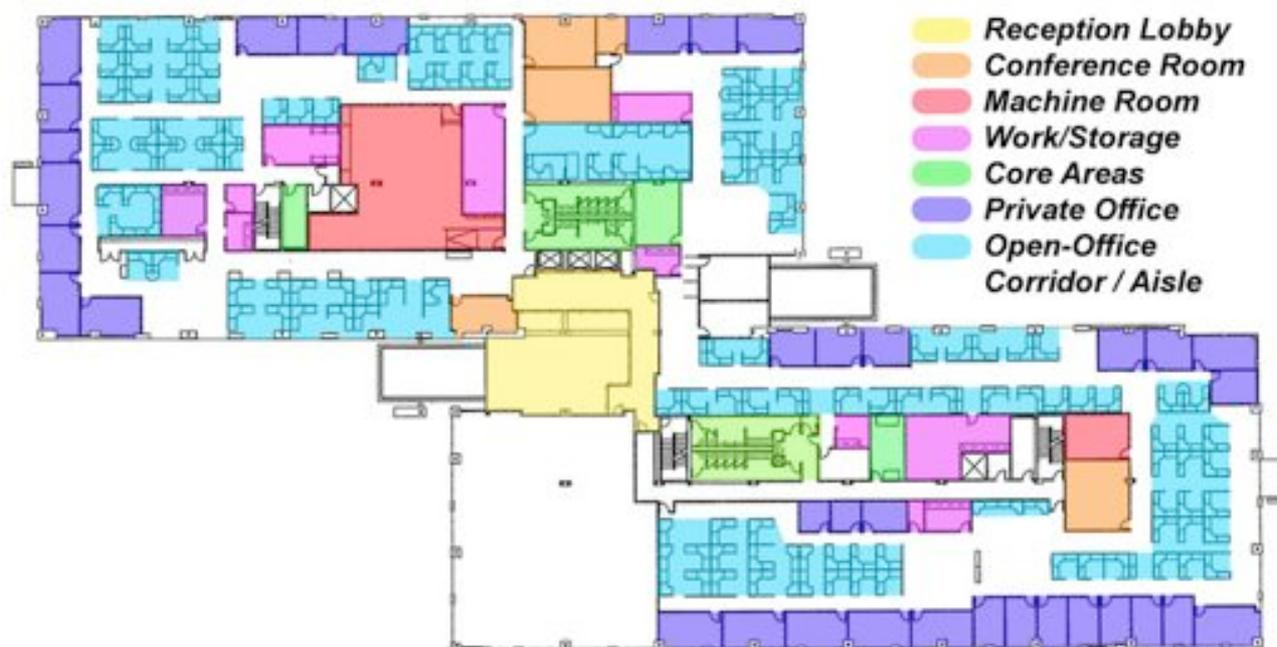
**Figure 1.** Floor Plan: Office Building Typical Floor Showing Types and Distribution of Spaces.
