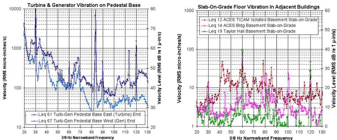
Charts 2 & 3 – Validation Measurements – Note that 30 Hz and 84 Hz Tones are Controlled<sup>6</sup>
