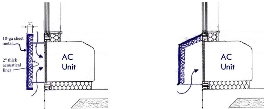
Figure 2: sections through air conditioner showing noise baffle (left) and hood (right) options
