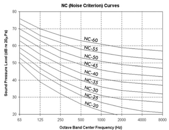
Figure 3. Noise Criteria-Allowable Noise
