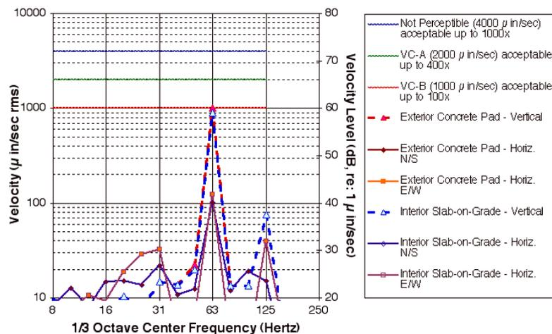
**Figure 4.** Existing Ground Borne and Structure Borne Vibration (1998)
